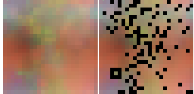
Figure 6. SOM visualizing 24 Bark bands of GarageBand loops, using mean amplitude (left) and the associative SOM, displaying black for non-associated nodes (right)
