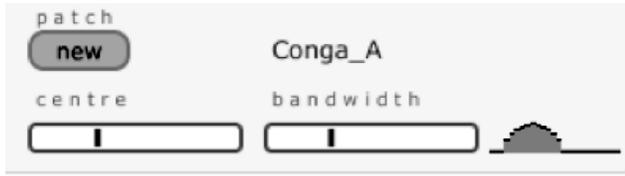
**Figure 2.** Defining a spectral band from which to choose a sample. Moving the sliders alters the displayed bandwidth to the right. Clicking on the “new” button will generate a random input vector from within the chosen bandwidth.
